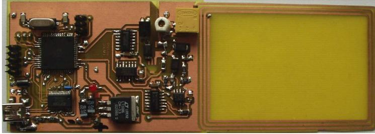
**Fig. 1.** Our stand-alone RFID emulation device.
